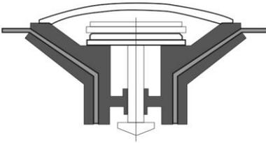
Overpressure valve protects the boat against unexpected pressure increase over the maximum working limit.
