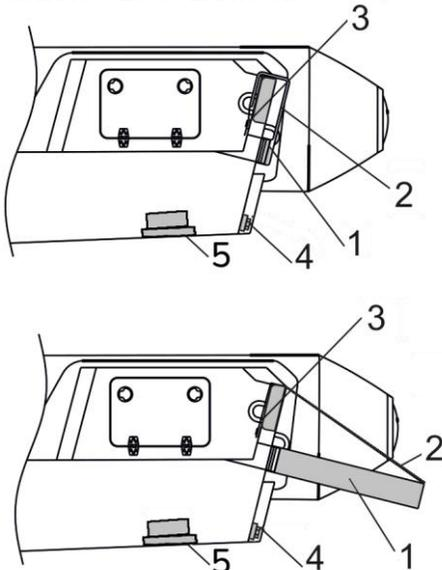
The boat's cockpit is self-draining. The drainage system has two drain hoses (1). To drain the water from the cockpit, disconnect the cord (2) of the hose (1) from the clamcleats (3) and straighten the drain hose behind the transom. After deck draining, reverse the steps. To pump water from deck below use the bilge pump (option 5), when the boat is in the water.
